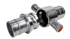
With rigged tails on each end of the coupling for a secure fit, with both male and female fixings for both ends, the instantaneous couplings are manufactured for Vigil Products. Commonly used by the fire brigade, they're also for general industrial use, agriculture and irrigation, and wash-down applications, the fire hose alloy couplings have a working pressure of 16 bar.
