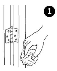
1. Open the door and thoroughly clean and dry the door and frame, ensuring that no grease or other residues remain.
