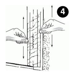
4. To ensure correct adhesion, rub your fingers firmly up and down the adhesive strips for 2 minutes. Then close the door and do not open for at least 15 minutes. If the above installation instructions of placement of strips at 3.5 cm and 5 cm from the corner of the door are not followed properly, a gap may result making the strips less effective, which may result in an accident.
