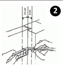
2. Close the door. Lightly draw with a pencil two vertical lines, one on the door exactly 3.5 cm from the corner, and one on the door frame exactly 5 cm from the corner, up to a height of 1.2 mtr from the floor.
