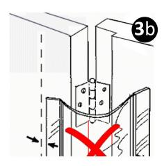
3a. Open the door at exactly 45 degrees and remove the protective paper from one adhesive strip. Attach the adhesive strip to the doorframe just inside the guideline, ensuring that the bottom of the strip is no more than 0.5 cm above the floor. Remove the protective paper from the second adhesive strip and attach it to the door. (See Drawing 3a and 3b)
